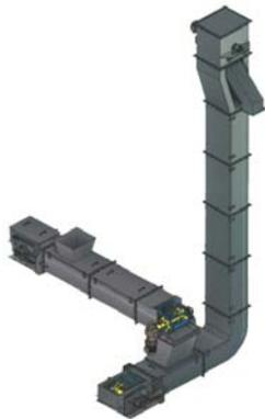
**WTW's** design of heavy duty, dust or gas tight, explosion-proof **Chain Conveyors (TKF)** are the most reliable and durable system available in any industry. Sticky, hot (up to 750° C), abrasive materials such as synthetic gypsum, alternative fuels and clinker are easily conveyed from 0 to 1,000 t/h, on single or double strand chains of 0.25 to 2 meters in width.
