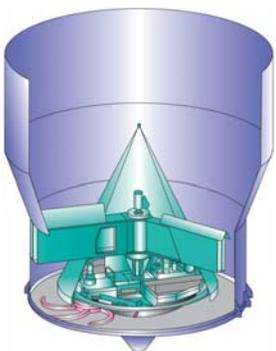
Our **Silo Discharger (PlanEX®)** is **WTW's** largest discharge system with material storage capacities up to 5,000 m<sup>3</sup> and silo diameters from 5 meters to 12 meters. It is the most effective in obtaining total mass flow of materials. The **Silo Discharger (PlanEX®)** is recommended in power, cement, wallboard, waster handling and other industries where non-free flowing materials have to be stored.
