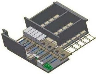
**Active Bottom Discharger (ABD)** can successfully store and discharge all types of lighter density bulk materials such as woodchips, bark, shredded tires, contaminated sawdust, garbage or other products with combustible properties. When considering alternative fuels to reduce your costs, we recommend you consider the use of a **WTW Active Bottom Discharger**.
