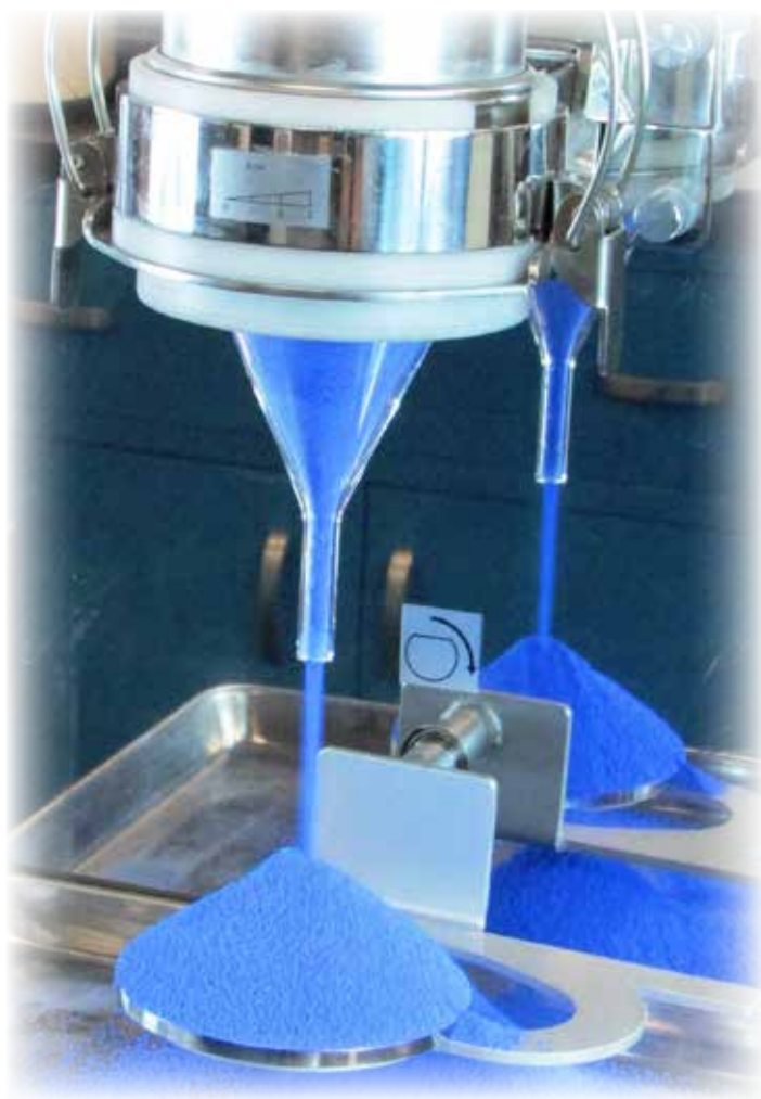
Angle of repose analysis on Micron Powder Characteristics Tester PT-X
