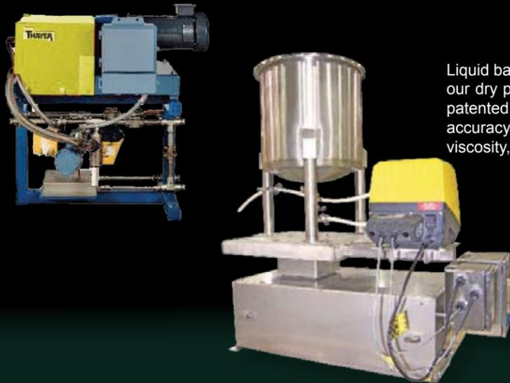
Liquid batch feeders utilize many of the same features as our dry powder Loss-In-Weight Feeders. Thayer Scale's patented FMSS technology scales are used to assure high accuracy and repeatable batching of liquids regardless of viscosity, pressure or temperature.
