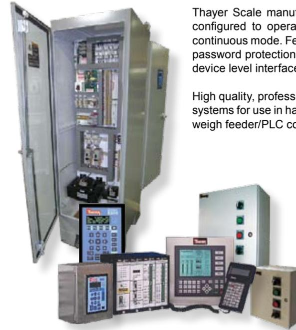
Thayer Scale manufactures a wide range of instrumentation products that can be configured to operate either a single or multi-feeder operation in either batch or continuous mode. Features include programmable analog and discrete I/O, multi-level password protection, RS232 and RS485 serial communications and a wide range of device level interfaces including DeviceNet, Profibus-DP, and Ethernet /IP.
