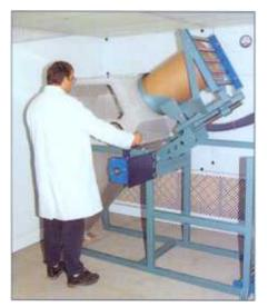
Hosokawa Vitalair manufacture a range of automatic and manual drum and keg tipping equipment designed to offer safe product transfer. Product tipping units can be integrated with downflow booths, laminar flow booths or be free-standing. Additionally they can incorporate glove box facilities and HEPA safe-change filters. (
