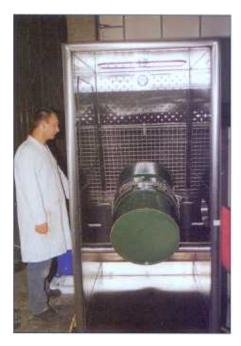
A controlled, once through, non turbulent air flow ensures good operator protection from dust and fumes. Individually designed to meet individual requirements the flow booths are usually supplied with integral fan/motor systems with equipment zoned according to area classifications.
