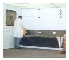
Designed with flush fitting panels and with no contamination prone crevices all our downflow recirculation booths are also available in non-standard sizes and layouts to suit customer requirements.
