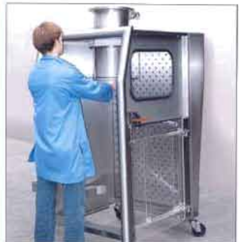
▲ Drum Filling in a Mobile Laminar Flow Cabinet with product exit door
