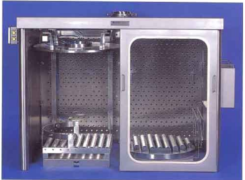
Laminar Flow Booth incorporating Keg Filling and Transfer Station ▲
