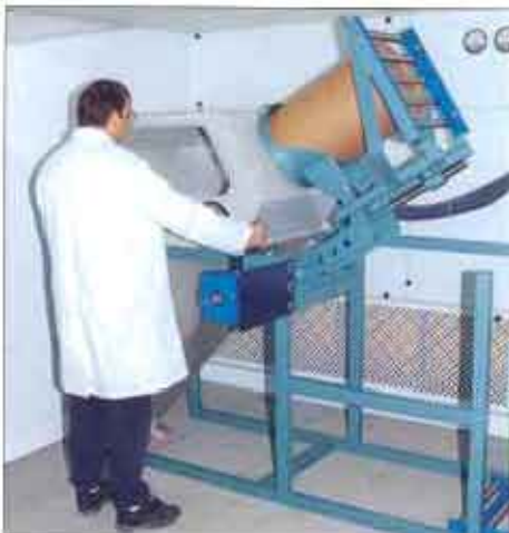
▲ Manual keg-tipping unit in a Laminar Flow Booth ▲
