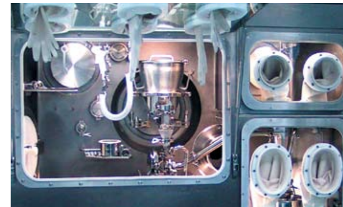
ALPINE SPIRAL JET MILL 100 AS WITH PHARMA-DESIGN METERING SCREW
