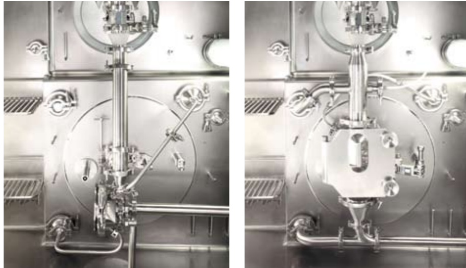
ALPINE SPIRAL JET MILL AS CAN BE EXCHANGED FOR ALPINE FINE IMPACT MILL UPZ
