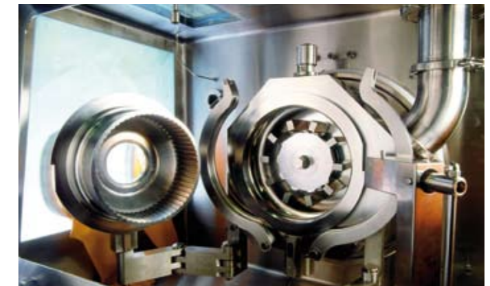
ALPINE FINE IMPACT MILL 315 UPZ FINE GRINDING ON A PRODUCTION SCALE
