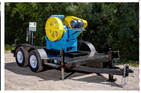
The PREMAC1 Mobile Access Crusher with sealed roller bearings provides reliable operation with minimal maintenance. High precision machining and assembly ensures smooth operation with minimal vibration. Anti-vibration mounting isolates crusher base from the support frame, thereby eliminating vibrations.
