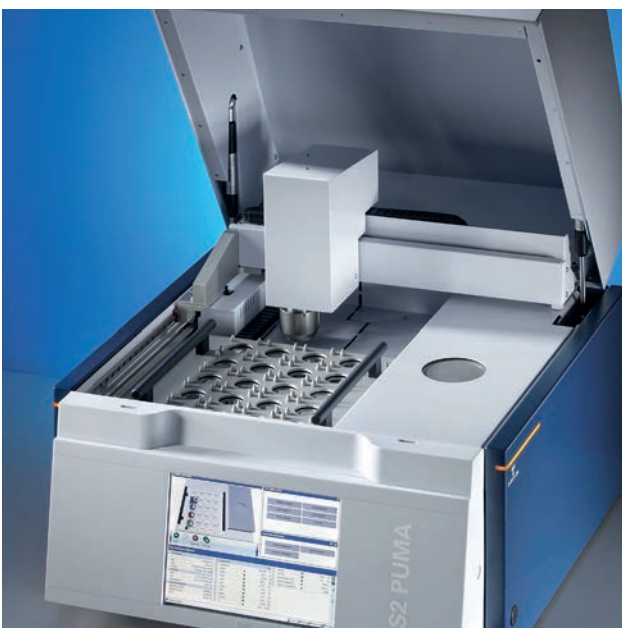
The XY Autochanger for high throughput
