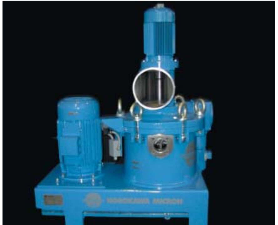
Mikro ACM 40 CL with direct classifier drive
