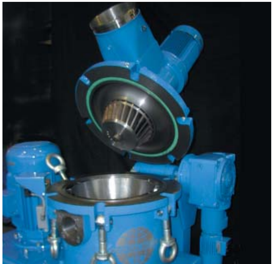
Mikro ACM 40 CL with opened grinding chamber cover
