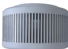
Fig.3 Classifying wheel made of alumina
