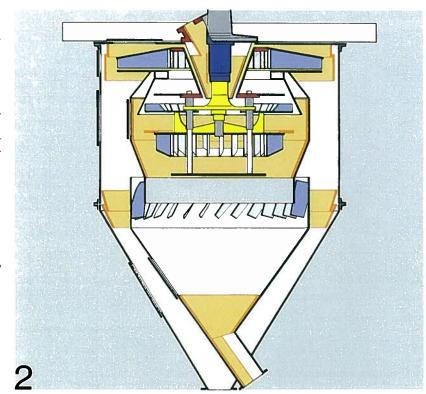
Orange and brown colour-coded components are designed as exchangeable wear-protection parts.
