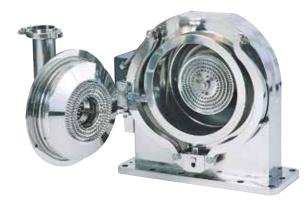
800 UPZ FINE IMPACT MILL WITH PLATE BEATER UNIT AND SIEVE GRATE PRESSURE-SHOCK-PROOF TO 10 BAR (g)
