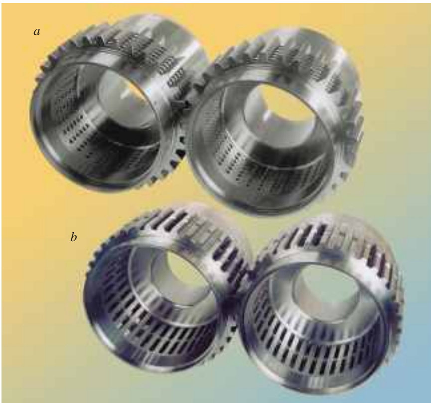
a Pair of rolls with press nozzles bored in solid extrusion rolls
