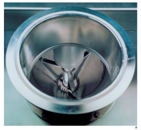
The combination of the rotor speed and screen selection determines the final particle size distribution (a, b). The critical gap between the rotor and screen can be adjusted manually or automatically. The rotor is designed for long life and maximum performance. Rotor seals are also available with air or Nitrogen purging.
