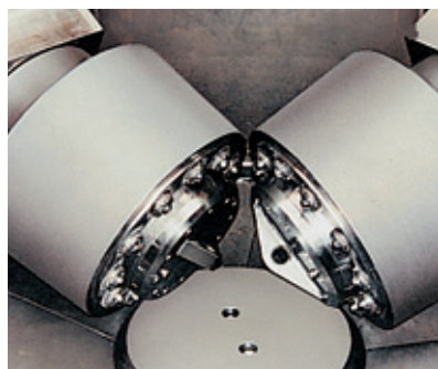
GRINDING ROLLERS AND GRINDING TABLE
