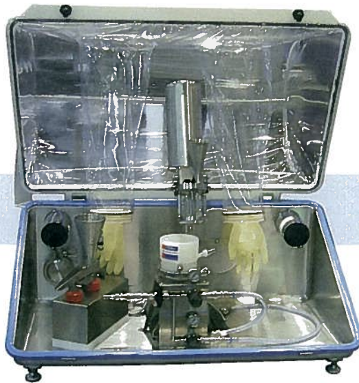
FLEXIBLE ISOLATOR (OEL < 10 µg/m³) WITH 50 AS IN PVDF
